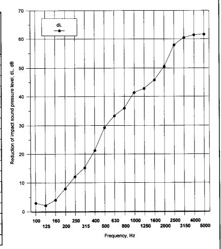
Ln,0: Is the normalised impact sound pressure level of the heavyweight bare test floor.
